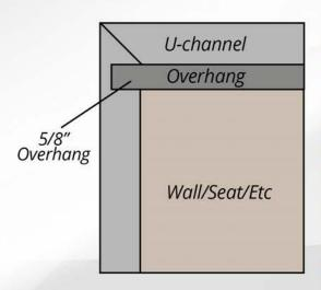
When building seats, benches or knee walls in a shower enclosure it is important to consider the overhang and try to keep it to an absolute minimum. Because of the metal U-channel that runs at the bottom of the shower glass, overhangs on seats and knee walls should never exceed 3/4", as that is the height of the metal U-channel.
